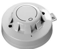
Not to be confused with the domestic CO detectors used in HMO type properties. These units, whilst not used very often, are for buildings where a traditional smoke detector cannot be used and a heat detector is not appropriate. They are not as effective as traditional smoke detectors and should be used as part of a fire detection solution and not the sole means of detection.
